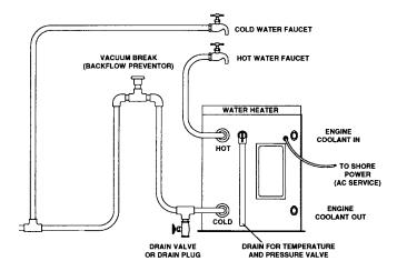
The "1700 Series" water heater provides hot water for galley and shower. Dense foam insulation provides better and longer heat retention than traditional fiberglass. The tank itself is protected by a 75 PSI T&P (temperature and pressure) relief valve. The cylindrical design of the tank enables it to withstand more pressure than a cube shaped tank.
